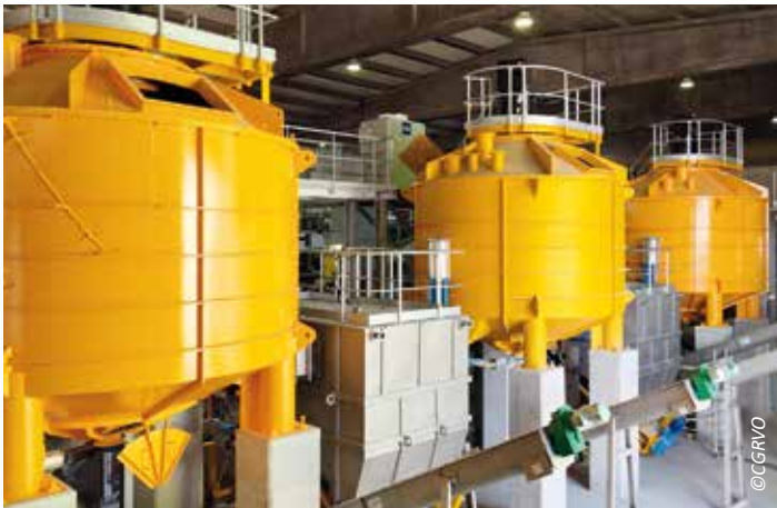
The 3x BTA Waste Pulpers as installed during the extension works in Granollers
